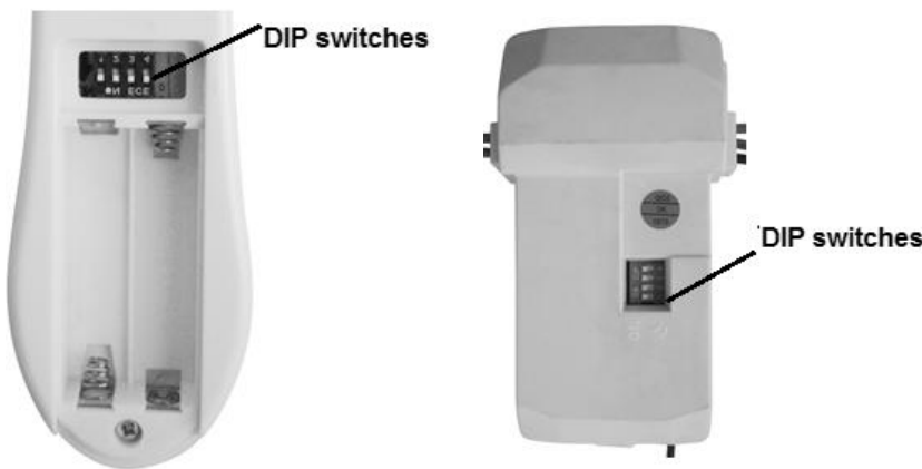
Fig. 11 Remote battery compartment
