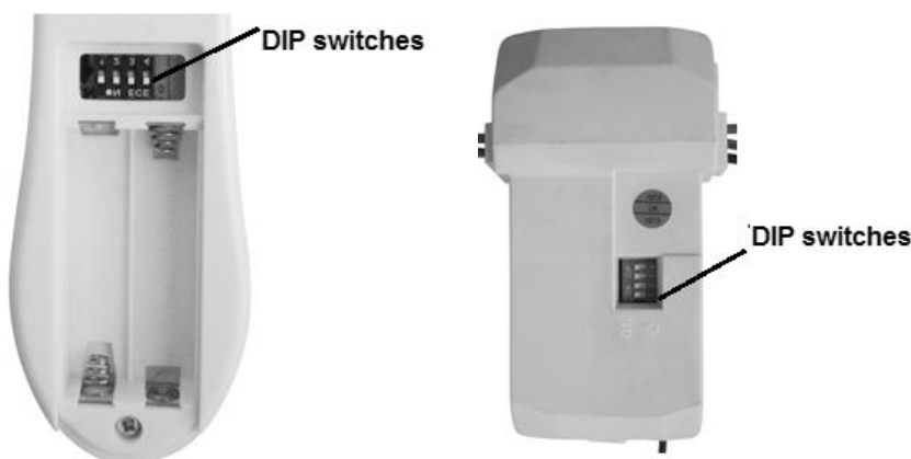
Fig. 12 Remote battery compartment
