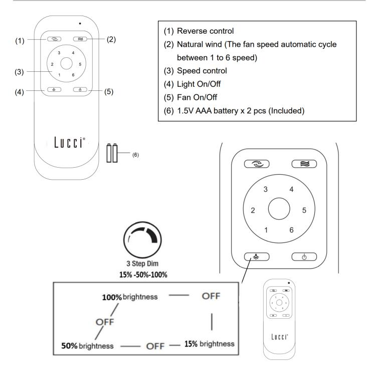
The remote has memory function. If the fan or light is turned off by the isolating switch, it will memorise and recover the last status when turned on next.
