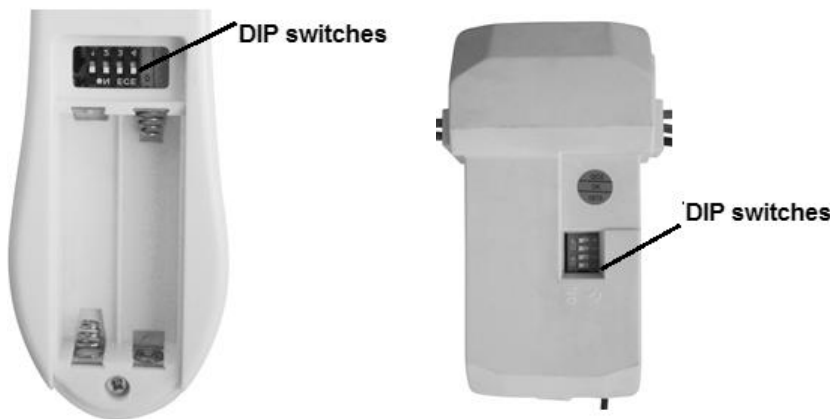
Fig. 11 Remote battery compartment
